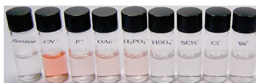
FIGURE 2. UV–vis absorption change of DNPA 1 ( 2.0 \times 10^{-5} M) in \text{CH}_3\text{CN} upon addition of 1.0 equiv of the anions and color change of DNPA 1 ( 5.0 \times 10^{-5} M) in \text{CH}_3\text{CN} upon addition of an equimolar amount of anions (from the left: 1 , \text{CN}^- , \text{F}^- , \text{AcO}^- , \text{H}_2\text{PO}_4^{2-} , \text{HSO}_4^- , \text{SCN}^- , \text{Cl}^- , \text{Br}^- ).
