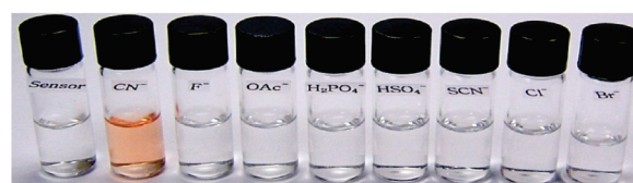
FIGURE 3. UV–vis absorption change of DNPA 1 ( 5.0 \times 10^{-5} M) upon addition of 2.0 equiv of each anion in \text{MeOH} – \text{H}_2\text{O} (10/1) and color change of probe 1 ( 1.0 \times 10^{-4} M) upon addition of 2.0 equiv of each anion in \text{MeOH} – \text{H}_2\text{O} (10/1) (from the left: 1 , \text{CN}^- , \text{F}^- , \text{AcO}^- , \text{H}_2\text{PO}_4^{2-} , \text{HSO}_4^- , \text{SCN}^- , \text{Cl}^- , and \text{Br}^- ).
